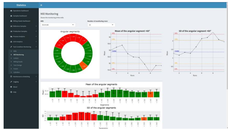
Figure 5: Dashboard of the PrepMaster Analytics showing the typical pattern of worn horizontal springs.
