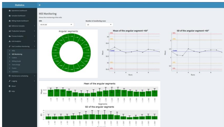
Figure 4: Dashboard of the PrepMaster Analytics used for TCM of the swing aggregate. For detection of deviations methods of statistical process control (SPC) are applied.
