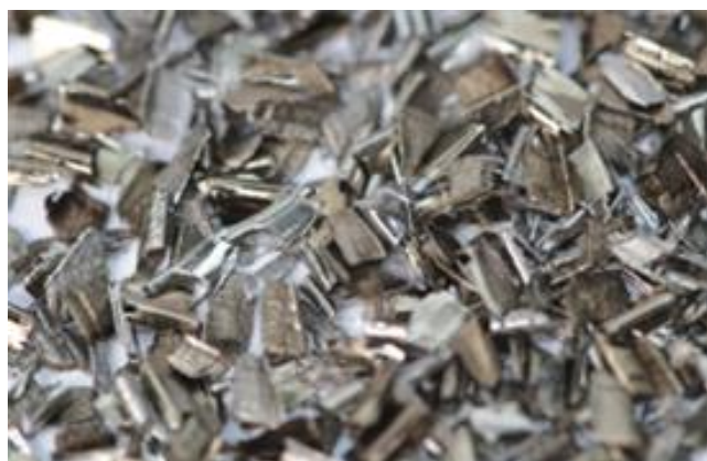
Figure 2: Typical aliquot of granular chips obtained from a steel sample showing the typical even, smooth and short morphology.
