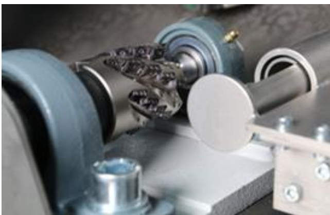
Figure 1: Cylindrical cutter module within the HS-F 1000 for production of granular chips
