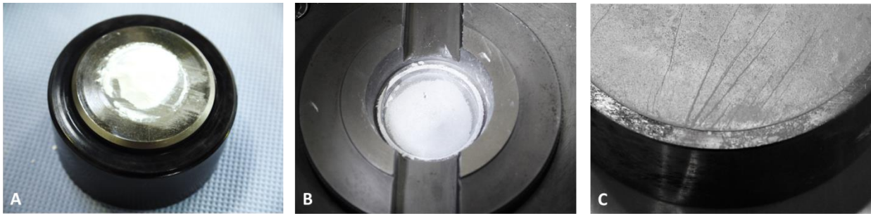
Figure 1: Miscellaneous sample preparation difficulties, when pressing strongly cohesive powders for XRF analysis:
