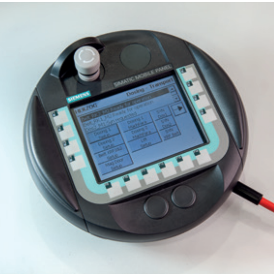
Central remote controller (optional for systems with several machines instead of individual control terminals at every machine)
