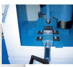
HPF with manual clamping device
