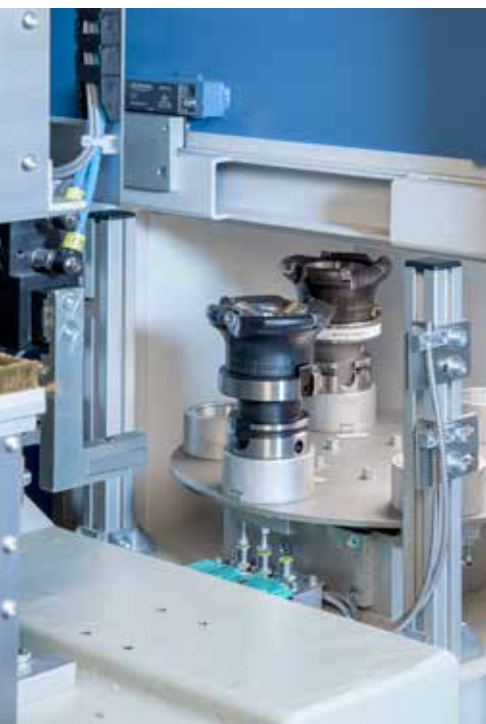
Automatic tool changing system for continuous operation without operator intervention.
